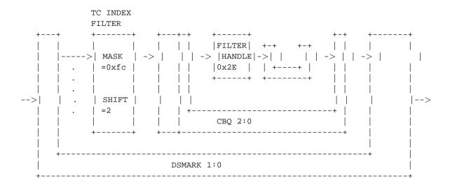
The packet arrives, then, set with 0xb8 value at DS field. As we explained before, dsmark qdisc identified by 1:0 id in the example, retrieves DS field and store it in skb->tc\_index variable. Next step in the example will correspond to the filter associated to this qdisc (second line in the example). This will perform next operations:
